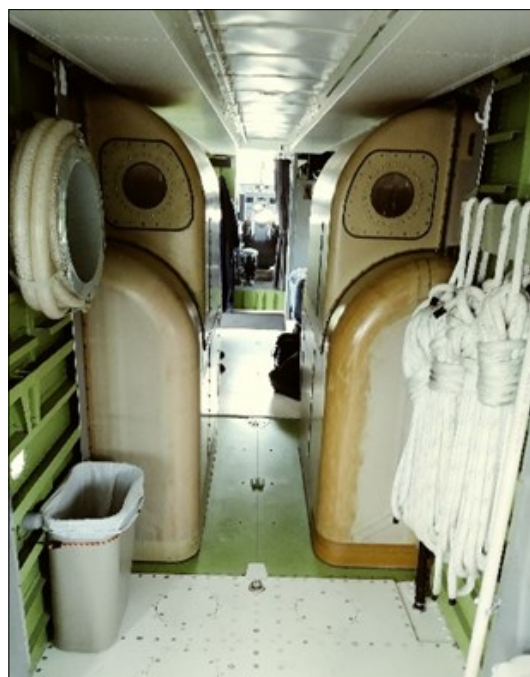
This CL-415 on the ramp at Yellowstone Airport can carry 1,600 gallons of water. See view of the water tanks from the interior of the plane in picture below.
